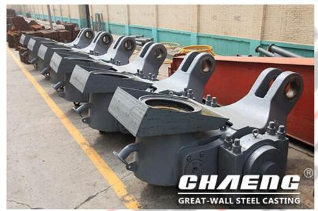
The vertical mill rocker arm produced by CHAENG is also one of the more important parts in the vertical mill grinding equipment, and each set of rocker arm also includes the upper rocker arm and the lower rocker arm, the central shaft , the bearing chock. And bearings, etc., which transfer the pressure of the hydraulic cylinder to the grinding roller, and then convert it into a grinding force on the bed.
