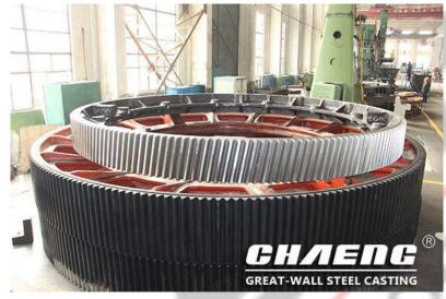
According to the load carried by the ball mill, or directly use the ball mill as a hollow simple bracket. It will use the discharge end as a fixed link support, and the discharge end can be used as a girth gear support; At this time, the ball mill is inflated and contracted freely by the feed end. If the pinion is mounted on the discharge port without being affected by the axial turbulence caused by the contraction, it will not cause extra and avoid axial friction or wear.
