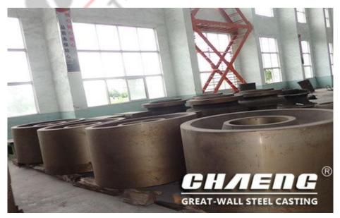
CHAENG is treated by normalizing and tempering in the casting of the supporting roller. The surface hardness of the outer circumference of the supporting roller is higher than 200HB, which greatly guarantees the quality of the rotary kiln supporting roller device.
