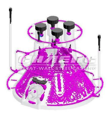
**Casting process two:** CHAENG adopts high-quality materials such as ZG230-450/GS-16Mn5/BS3100B2 which can make the cast slag pot have good plasticity and high melting point;
