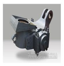
Swing Lever is one of the major components of vertical roller mill. The rocker device is mainly composed of upper rocker, down rocker, rocker arm shaft, bearing, bearing seat etc. The upper rocker arm used to install the roller, the down rocker arm connects with hydraulic system. Two rocker arms are connected into a whole by shaft, taper sleeve and taper pin.
