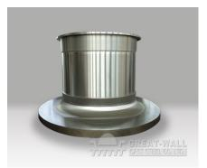
Trunnion Bearings is an important part loading mill cylinder rotary. These casting surfaces such as the neck contacted with the mill spherical tile and the circular arc neck contacted with cylinder are free of blowhole and sand inclusion in the cast process; the position parts contacted with spherical tile need to grinding after machining in machining process. So that can ensure the tolerance and roughness. So the products requirement is very
